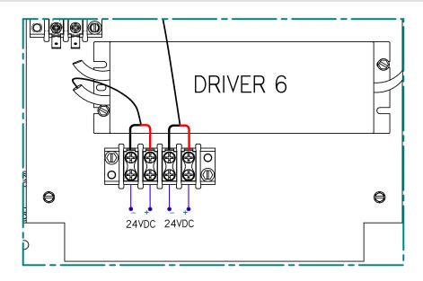
6. If the voltage reading at the drivers output is 0 VDC, then the LED driver is either incorrectly wired or faulty. Ensure that the ground, neutral and line wire from the driver is correctly wired to the respective terminals on the driver's input. If the driver is correctly wired and the LEDs do not power on, the driver is faulty. Submit an FQR or contact your local Price representative for replacement LED drivers.
