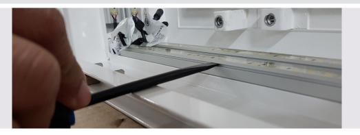
**Step 3:** To install the new LED strip, ensure the connector ends on the LED are oriented such that the male connector of one LED and the female connector of the adjacent LED align.
